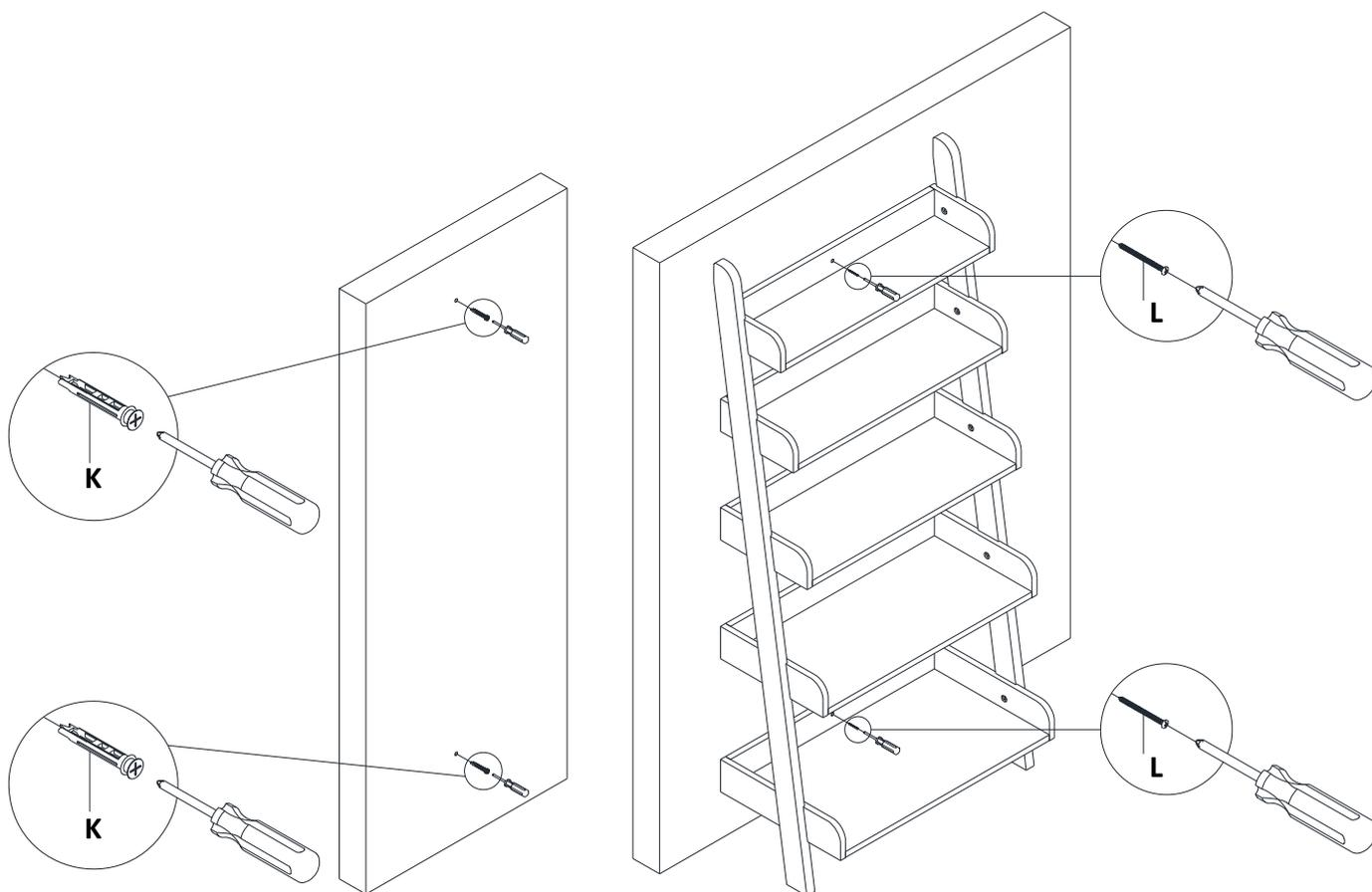
**For stud mounting:** Use a screwdriver to secure the Shelf through Wood Screw (M) at the marked locations, simply drive down Wood Screw (Y) for securing.
