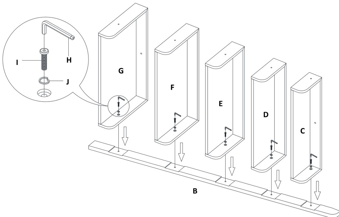
2. Attach the remaining leg (A) to assembly as shown. Insert Bolt (I) thru Spring Washer (J) , securely tighten all bolts with the Allen Key (H).
