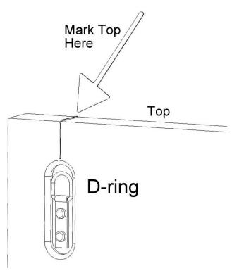
pencil mark you made on the top edge does align with the D-ring. Repeat this step with the other panels so that each panel has two pencil marks on the top edge which align with that panel's D-rings.
