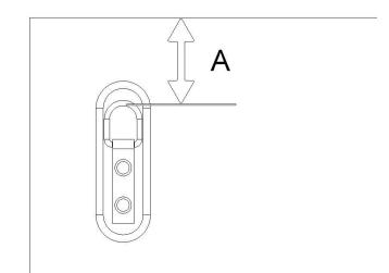
midpoint. The horizontal line will be used as a guide to hang the panels with the upper panels 3, 4 being mounted above the horizontal line and the lower panels 1, 2 being mounted below the horizontal line. The horizontal line should be about 64 inches long.
