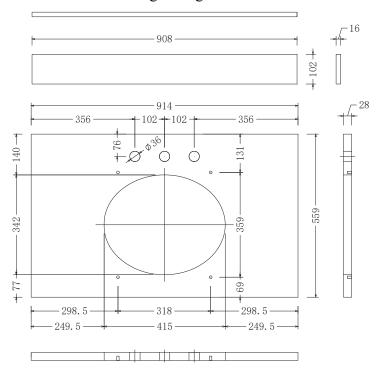
249.5mm = from side of marble top to side of basin 458mm = from side of marble top to basin drain hole 248.5mm = from front of marble top to basin drain hole 77mm = from front of marble top to front of basin 310.5mm = from centre of basin drain hole to back of marble top
