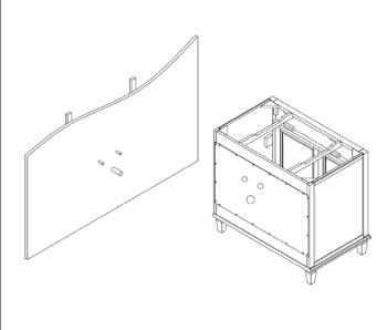
Install proper mounting hardware in wall. Attach vanity to wall.
