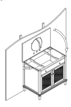
Wipe off excess Sealant Let Sealant cure according to manufacturer's directions before installing plumbing fixtures. Apply Sealant
