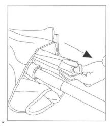
2. One hand holds rib, while one hand pulling pocket, to set each Rib End into each pocket.(Fig 2-1/2-2)
