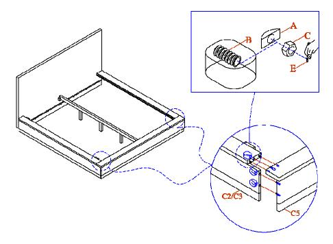
6. Put slat roll (C6) between side rails (C2/C3).
