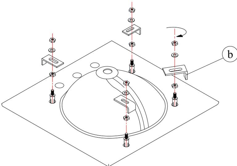
Note: Before installing marble top onto console base; console needs to be properly leveled, shimmed (if necessary), and secured to floor and wall as required.
