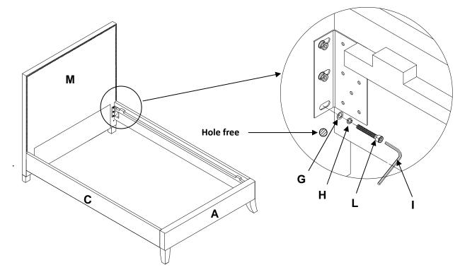
Date: 10-Oct-14 Rev: 3. Place the Slate (D) on the bed, fix with screw (J), and then tighten with Phillips Head Screwdriver. Fully tighten the bolts in step 2 with Allen key (I). Assembly is complete.
