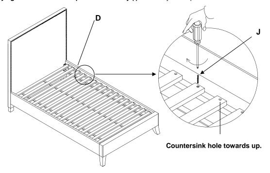
4. This headboard could assemble with the Metal bed frame (sold separately) as below:
