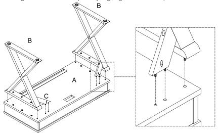
3. Insert the Flat Washer (E), Lock Washer (F) and Allen Bolt (G) into the pre-drilled holes on both legs. Use Allen Key (H) to secure. Insert the wood screw (I) into the angle blocks (C). Secure with a Phillips head screwdriver. **Do not tighten bolts and screws.**
