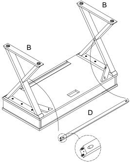
5. Secure the stretcher (D) to the leg (B) with wood screw (I), but do not tighten.
