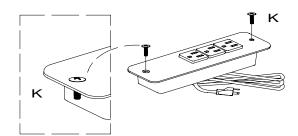
9. A panel with grooves for cords is held by a magnet under the top back. Take panel out to access the cut-out behind. Insert the Cord Set (J) with Screw (K) into the cut out and the predrilled holes.
