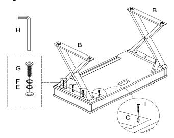
4. Attach the stretcher (D) between the X-Leg (B) by inserting the dowel into the pre-drilled hole.
