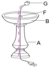
2. Put the submersible pump (G) inside the basin (B) of the fountain. Then insert its electrical wire into the hole of the pipe (F) that is on the inner part of the basin (B) of the fountain. Thread the electrical wire through the body of
