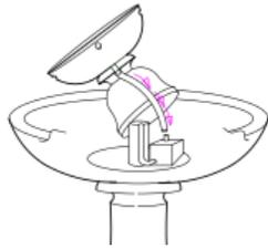
3. Put the top tier (C) of the fountain and connect the flexible hose (E) to the spout of the submersible pump (G). Make sure the flexible base (E) is connected tightly to the submersible pump (G) then place the top tier (C) on the basin (B) of the fountain.
