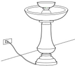
4. Put 4 litres of water inside the basin (B) of the fountain then Plug the male plug into the outlet.
